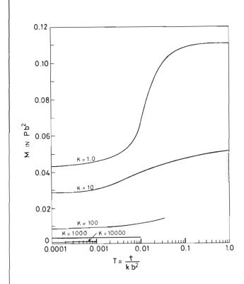
FIG. 4 EFFECT OF MEMBRANE TENSION ON THE MOMENT
