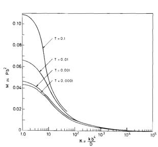
FIG. 3 EFFECT OF FLEXIBILITY INDEX ON THE MOMENT
