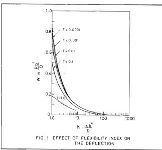
equivalent membrane tension on moments and deflections is more pronounced for such loading. This is true because the moments in uniformly loaded plates resting freely on a subgrade without shearing forces is equal to zero and the deflections of such plates are uniform. Plates with concentrated loads were studied to find the effects of the parameters on more practical cases.
