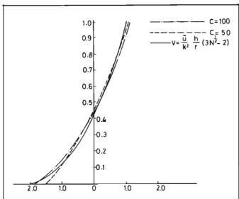
Fig. 1 RADIAL VELOCITY DISTRIBUTION ACCORDING TO EQUATIONS 5 and 6
