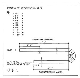
The total energy loss in the curved channels, was measured at established sections, A and A', in Fig. 3. Sections A and A' were established on the basis that, the hydraulic structure of the flow, at these sections is independent of the bend. Longitudinal velocity distributions have returned to normal, and no induced spiral motion by the bend appeared at these sections. This was verified by experiments.
