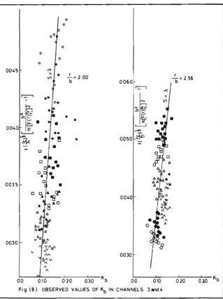
$$K_{b} = \frac{\lambda}{\pi} \left[ \left( \frac{r_{c}}{h} \right)^{\frac{1}{3}} - \frac{b^{2}}{r_{c} \left[ F(r) \frac{r_{o}}{r_{i}} \right]^{2}} - 1 \right] \dots (21)$$
