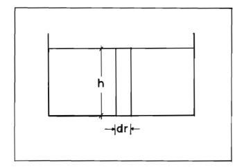
Considering an area-element of width dr and height h, the average discharge passing through this element may be given by:
